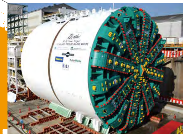
Ø17.45 m EPB TBM (United States)
