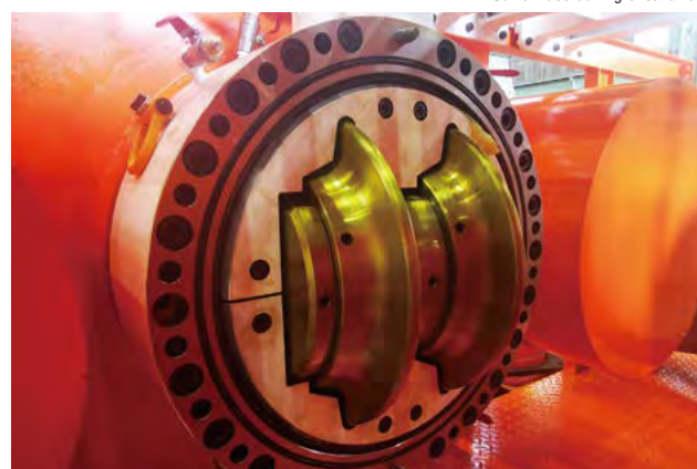
Cutter frame interior during cutter exchange
