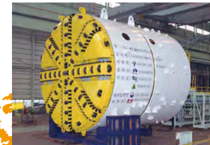
Ø7.8 m Slurry TBM (South Korea)
