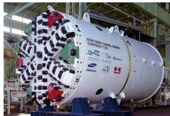
Ø5.22 m EPB TBM (United Arab Emirates)
