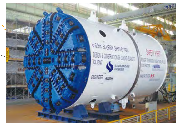
Ø6.9 m Slurry TBM (Singapore)
