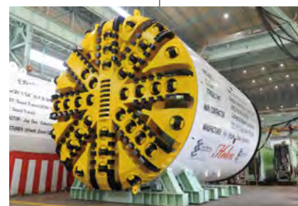
Ø6.44 m Slurry TBM (India)
